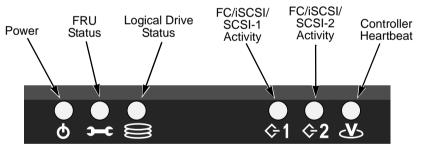
Figure 1. VTrak M500f/i/p front panel LED display
